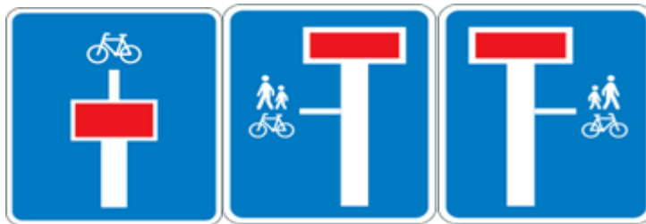
Fig. 2. Examples for the traffic sign "A dead end, except for cyclists and pedestrians" used in Denmark
