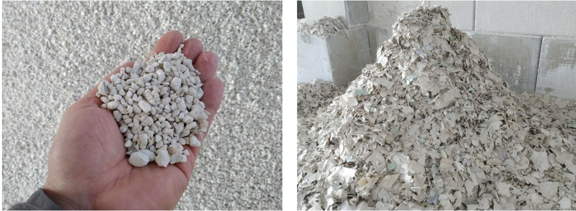
Fig. 38. Products of the processing of gypsum plasterboard: Gypsum grains (left) and cardboard flakes (right)
