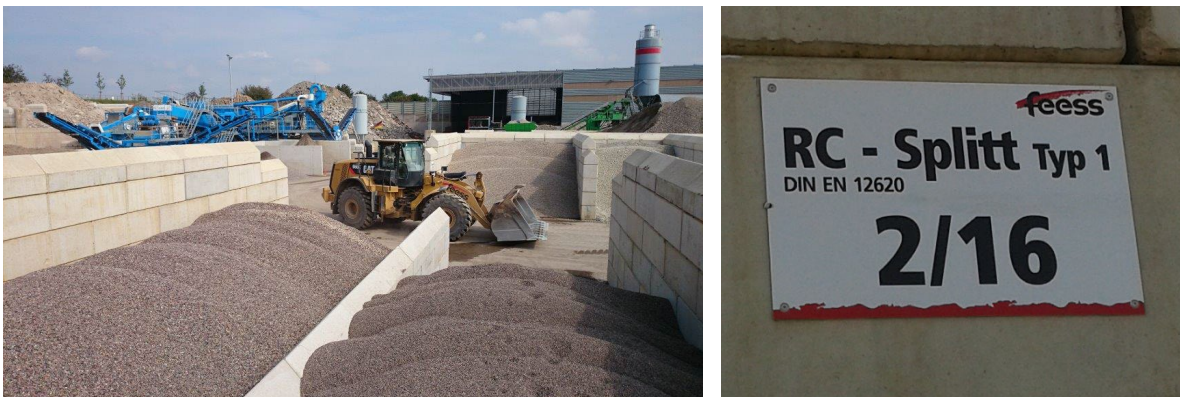
Fig. 15. Box storage of recycled building materials and labelling
