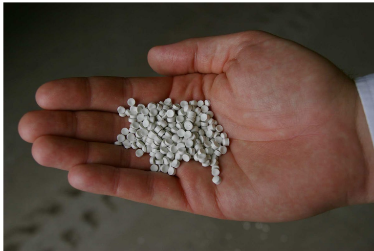
Fig. 50. Processed PVC from window frames [33]
