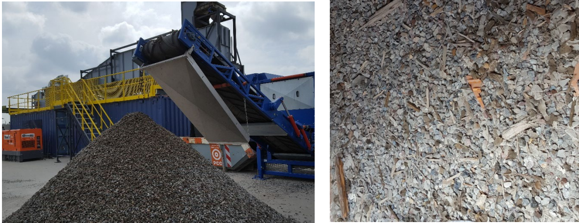
Fig. 27. Air shifter for separation of lightweight materials, cleaned heavy material separated lightweight (left), lightweight materials (right)
