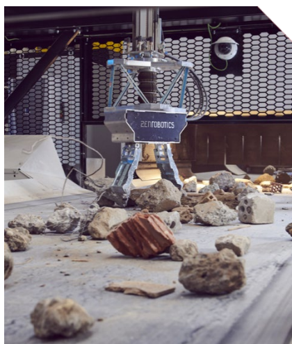
Fig. 29. Heavy picker sorting construction and demolition waste [17]
