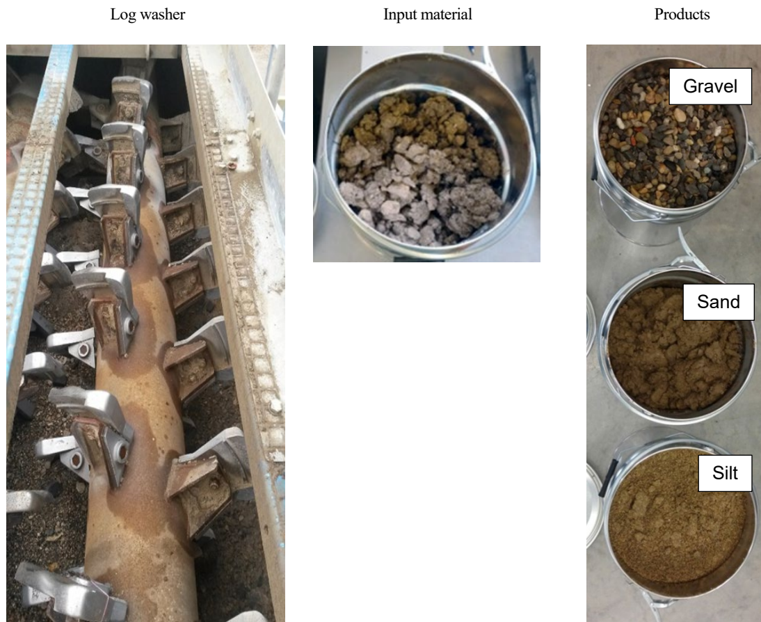
Fig. 44. Log washer, input material and products from the whole cleaning process
