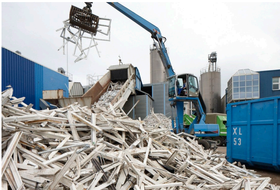
Fig. 48. Feeding the material into the first shredder [32]
