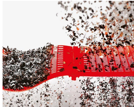
Fig. 18. Functionality of a flip-flop and example for the movement of the material [13]
