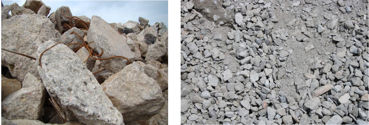
Fig. 23. Feed material concrete rubble (left) and produced recycled aggregates 0/45 mm (right)
