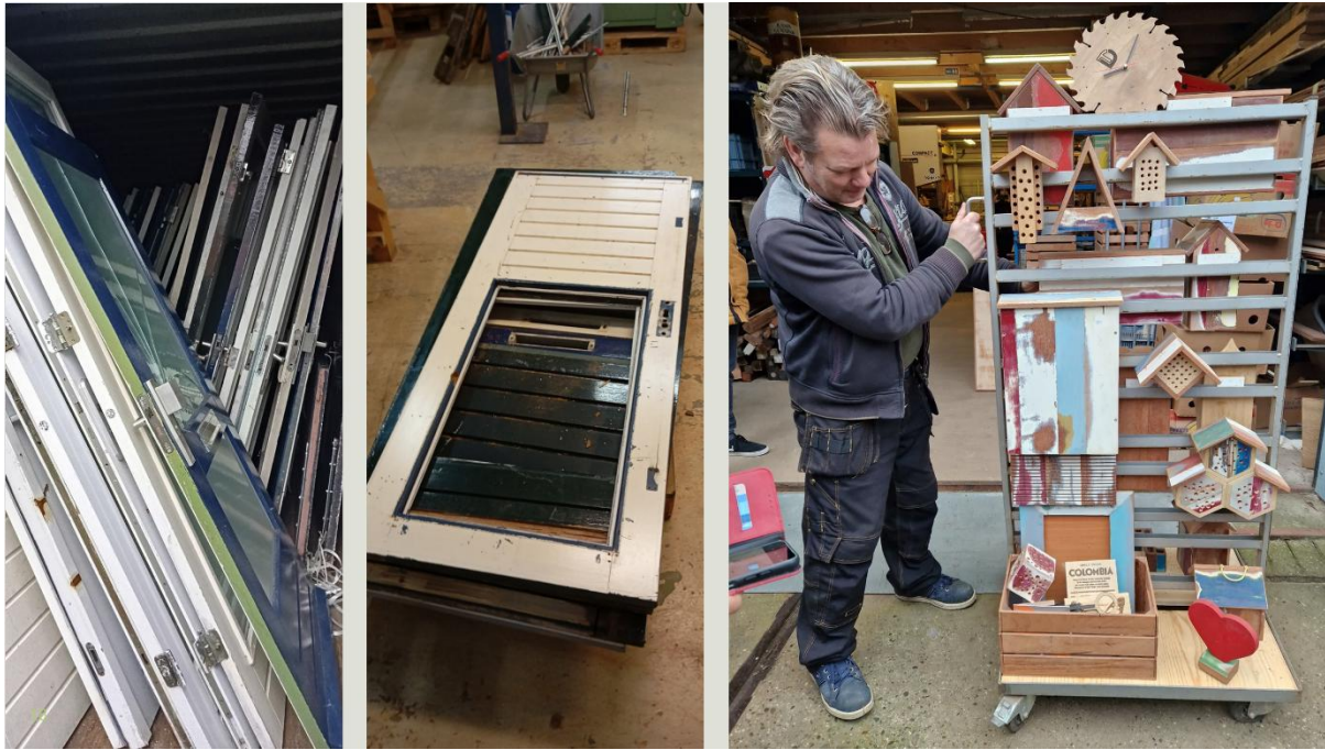
Figure 2: Door remanufacturing process at De Terugwinning. Left, container filled with collected doors. Middle, doors with metal and glass elements removed. Right: Exhibitor of products made from leftover wood from the remanufacturing process.
